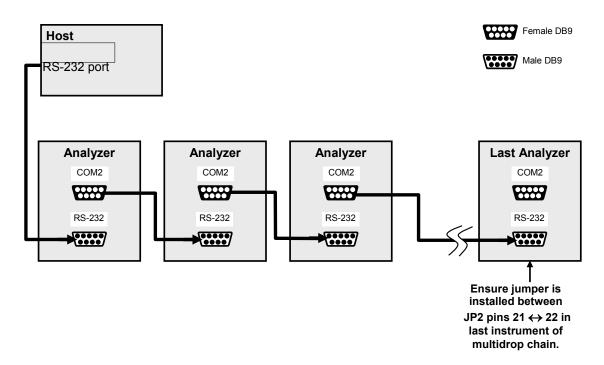
Figure 3-17: RS-232-Multidrop PCA Host/Analyzer Interconnect Diagram
